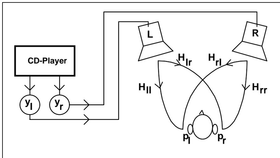
Fig. 2 – Scheme of the loudspeakers-ears transfer functions
