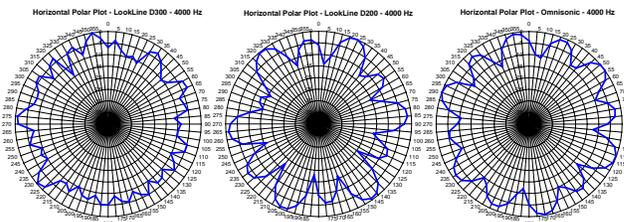
Fig. 45 – directivity patterns at 4 kHz
