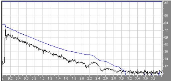
Fig. 25 – octave-band filtered IR with silenced pulsed event
