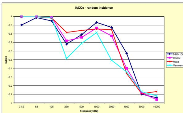
Fig. 52 – IACC measured with the 4 dummy heads
