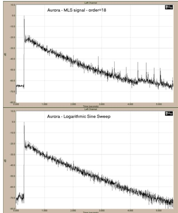
Fig. 7 – comparison between MLS and sine sweep measurements
