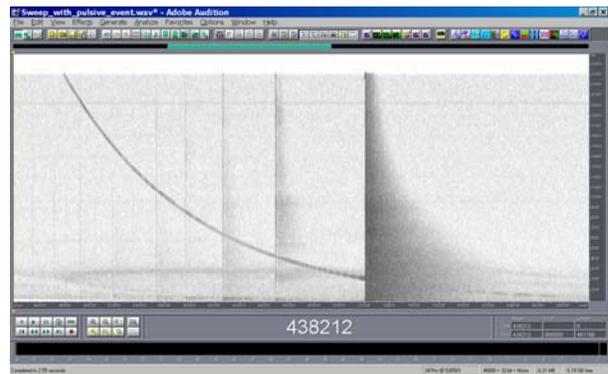
Fig. 24 – effect of the silenced pulsive event on the deconvolved IR
