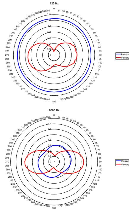
Fig. 50 – ST-250 – polar patterns at 125 Hz and 8 kHz
