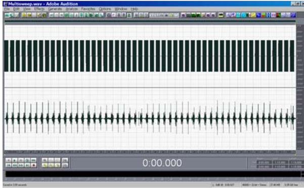
Fig. 38 – multisweep signal (test and response)
