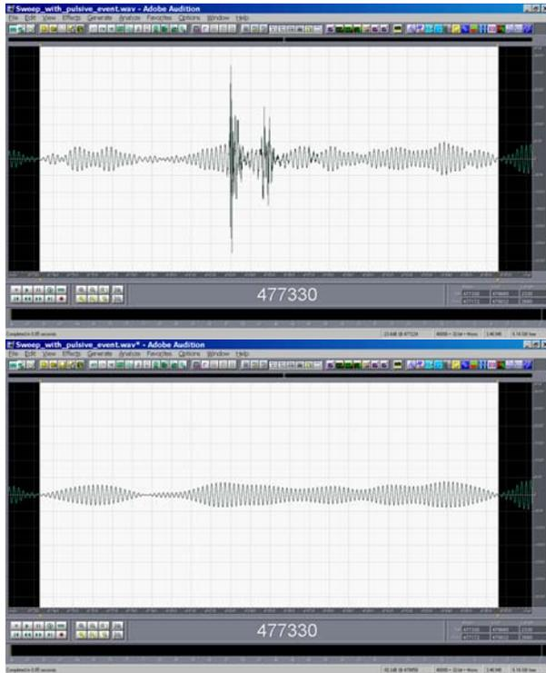
Fig. 29 – effect of FFT filter for removing the pulsvie artifact
