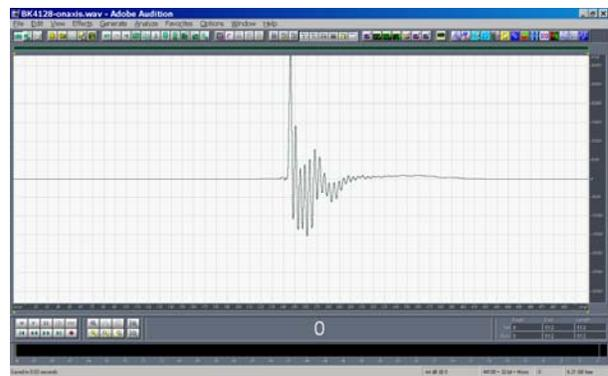
Fig. 15 – measured IR of the artificial mouth system
