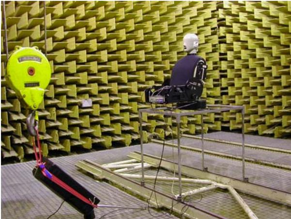
Fig. 51 – anechoic measurements on dummy heads
