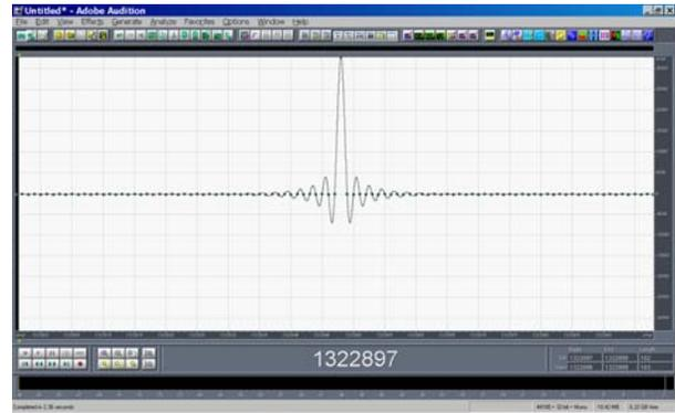
Fig. 9 – reduced pre-ringing artifact without fade-out
