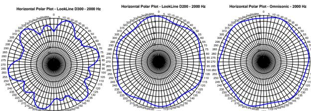
Fig. 44 – directivity patterns at 2 kHz
