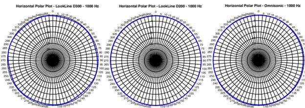
Fig. 43 – directivity patterns at 1 kHz
