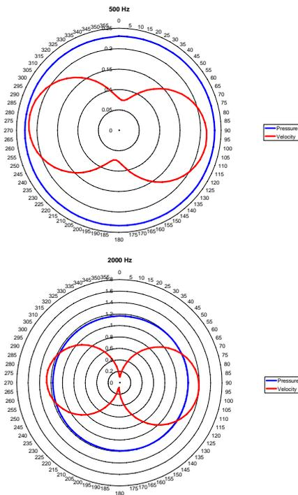
Fig. 49 – ST-250 – polar patterns at 500 Hz and 2 kHz
