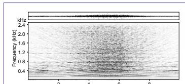
➤ 7-meter inflatable boat with 130 HP in-outboard engine (20 knots speed) recorded at a distance of 10 meters ( $L_{\text{Leq}, 1\text{min}} = 130.4 \text{ dB re } 1 \mu\text{Pa}$ ).
