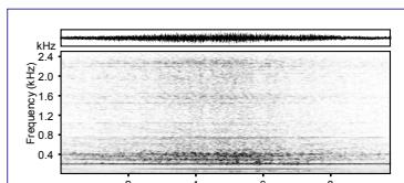
➤ 5-meter fibreglass boat with 40 HP outboard engine (15 knots speed) recorded at a distance of 10 meters ( $L_{\text{Leq}, 1\text{min}} = 129.6 \text{ dB re } 1 \mu\text{Pa}$ ).
