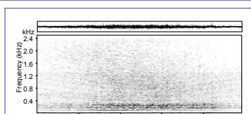
➤ 8.5-meter cabin cruiser with 163 HP inboard diesel engine (6 knots speed) recorded at a distance of 10 meters ( $L_{\text{Leq}, 1\text{min}} = 131.8 \text{ dB re } 1 \mu\text{Pa}$ ).
