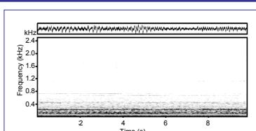
➤ 340-meter cruise ship with diesel engine (5 knots speed) recorded at a distance of 6 nautical miles ( $L_{\text{Leq}, 1\text{min}} = 108.1 \text{ dB re } 1 \mu\text{Pa}$ ).
