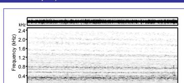
➤ 26-meter tourist ferry with inboard diesel engine (6 knots speed) recorded at a distance of 10 meters ( $L_{\text{Leq}, 1\text{min}} = 152.2 \text{ dB re } 1 \mu\text{Pa}$ ).
