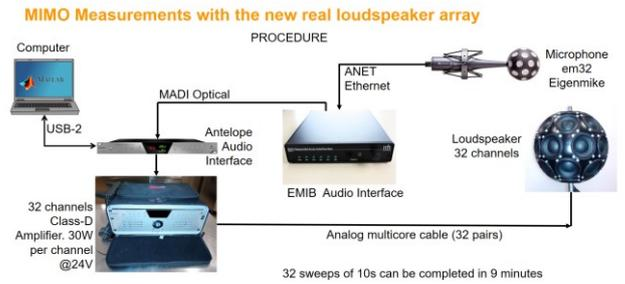
Fig. 5. Setting of the measurement chain.
